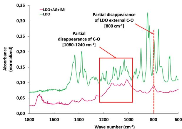
Fig. 1 FTIR analysis of a neatly synthesized LDO and a polymerized LDO/GA system.
