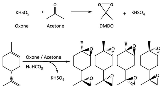
**Scheme 2** Epoxidation of (*R*)-(+)-limonene with *in situ* generated DMDO from Oxone/acetone.
