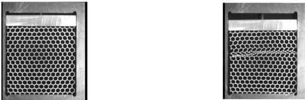
Fig. 1 Compression of a circular honeycomb in a staggered stack
