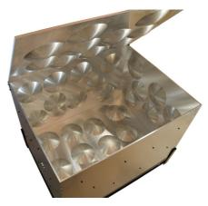
**Fig. 3** Photograph of the chaotic RC at INPHYNI with length L=100 cm, width W=77 cm and height H=62 cm. At the walls 54 spherical caps of radius  $r_c=10$  cm and cap height  $h_c=3$  cm are used. The total internal volume is V=0.451 m<sup>3</sup>.
