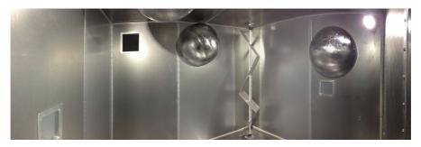
**Fig. 1** 180-degree photograph of the chaotic RC at ESYCOM. The commercial RC consists in a rectangular metallic cavity of dimensions W = 2.95 m, L = 2.75 m and H = 2.35 m and was modified by placing 3 hemispheres with radii of 40 cm (one at the ceiling and two on adjacent walls). The mechanical stirrer in the far corner can be seen.
