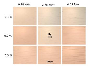
**Fig. 2** Snapshots of the suspension microstructure at the fixed elapsed time t = 20 min and different intensities H (or  $H_0$ ) of the applied magnetic field and different particle volume fractions  $\varphi$  (reprinted from Ezzaier et al. J. Chem. Phys. **146**, 114902 (2017) with kind permission of American Institute of Physics).
